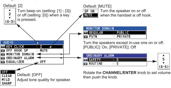
Rotate the **CHANNEL/ENTER** knob to select [AUDIO] on the [MENU] screen then push the knob.
